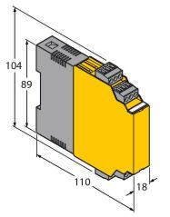
Isolating switching amplifier, 2-channel; 2 transistor outputs; input NAMUR signal; selectable ON/OFF mode for wire-break and short-circuit monitoring; switchable between NO / NC mode; removable terminal blocks; width 18 mm; universal voltage supply unit
