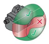
The left figure shows how the read/write head must be aligned towards the data carrier. As an example here the read/write head TNSLR-Q42TWD-H1147 is shown (instructions valid for all suitable read/write heads).
